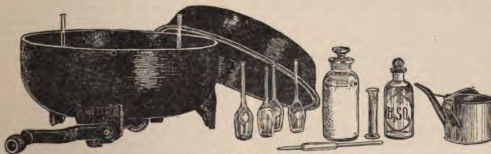
Fig. 168. Babcock test outfit.
